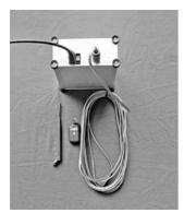
There is a SMA socket on the right side for the antenna, marked "RF".
