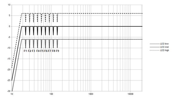
It is advised to first measure the microphone spectrum with the amplifier in pink/white or external in ""E"" setting, and take a note on which third octave bands need level adaptation. You will notice that the output level in ""E"" is always 6dB lower than the ""L"" and ""A"" settings. This is needed for protection of the sound source.
