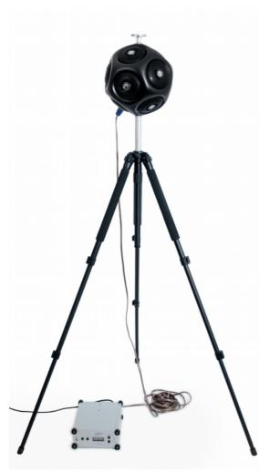
The Qam measurement amplifier is designed to power sound sources and electro-dynamic shakers. The amplifier is intended for indoor use, but can be used outdoors as long as it is protected against rain, excessive dust, etc.
