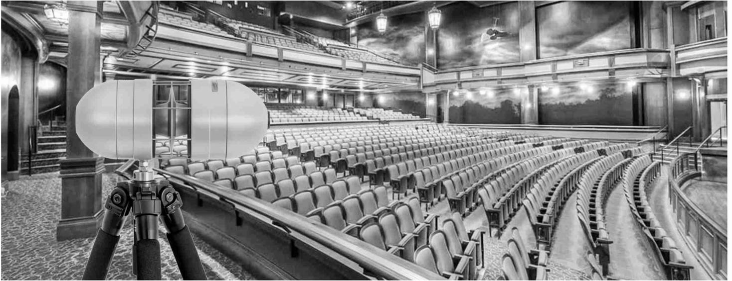
**Qoms<sup>2</sup> is highly accurate at a maximum sound power level of 110 dB and shows an omnidirectional pattern over large frequency bands.**
