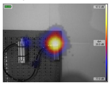
The device's 176 microphones increase the sensitivity and dynamic range: the result of a conventional acoustic camera with around 70 microphones can be seen on the left. The large leakage is detected, but the smaller leakage is not. It disappears in the acoustic fog due to the limited dynamic range. More microphones improve the sensitivity and dynamic range. On the right is the result of the Ultra 3. The large and small leaks are visible. Even at 20 dB dynamic range, no acoustic fog is visible.
