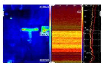
Measurement of a compressed air leak. The acoustic image can be seen on the left and the thermal image on the right.
